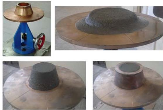
Figure (2): Flow table for mortar workability
