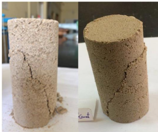
Figure (4): Mode of failure
