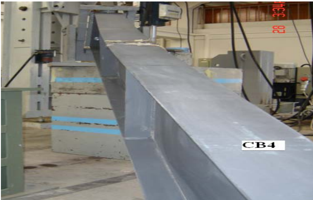
Figure (12): Lateral-Torsional Buckling Mode of Beam CB4.
