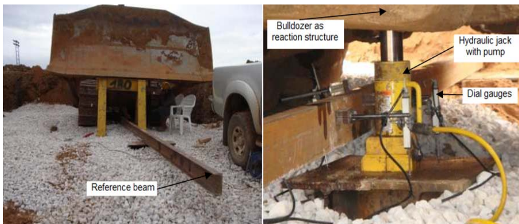
Figure (6): Load test on stone column
