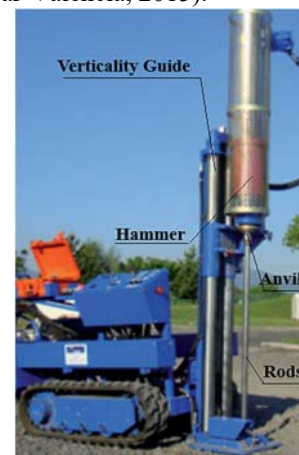
Figure 1. Photo illustrating a typical DPT test device
