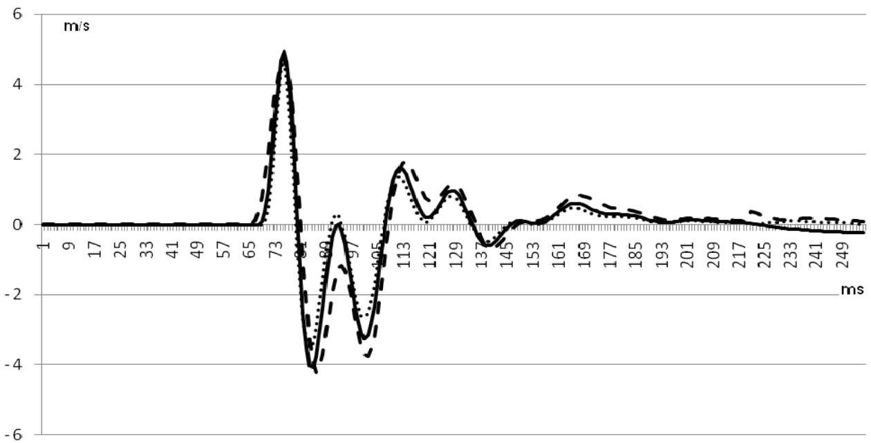
Figure (5): Velocity of rail in wheel flat point for different velocities 300km/h _____ 250km/h - - - - - 200km/h .....
