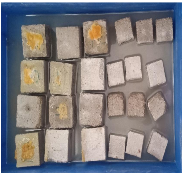
Figure 4. Mortar samples immersed in sulphuric acid solution
