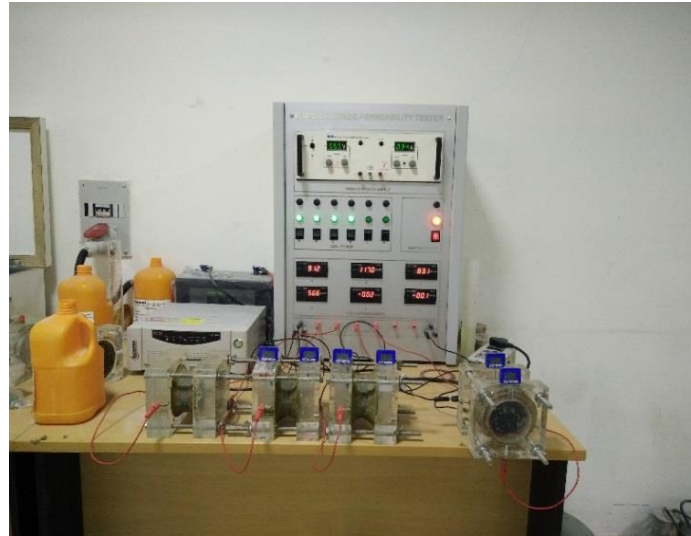
Figure 7. RCPT test setup
