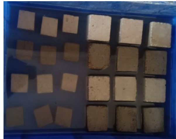
Figure 5. Mortar samples immersed in sodium sulphate
