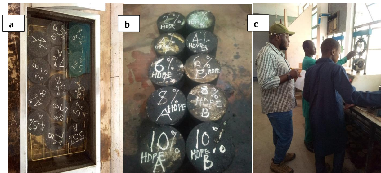
Figure (3): Experiment process (a) Threshold sample curing (b) HDPE-modified sample and (c) Marshall testing setup
