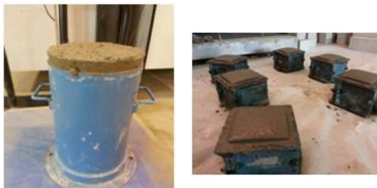
Figure (4): Photograph showing the swelling of concrete samples
