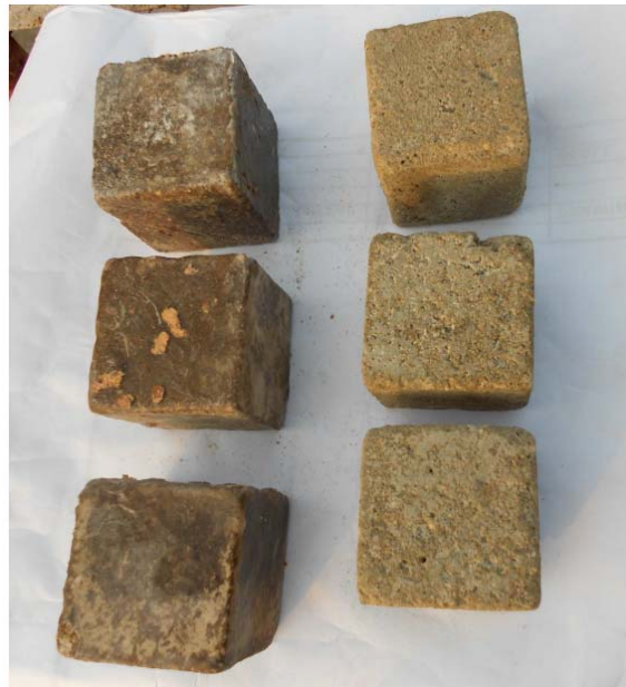
Figure (2): Specimen placed in ambient environment (left: single layer of resin, right: controlled)
