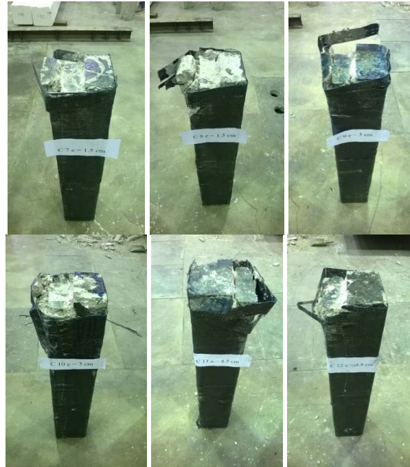
Figure (14): Failure modes for rehabilitated specimens
