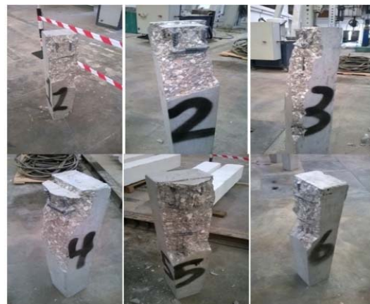
Figure (13): Failure modes for control specimens
