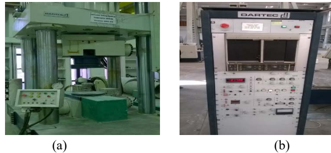
Figure (6): Testing machine (a) hydraulic jack and (b) data acquisition system
