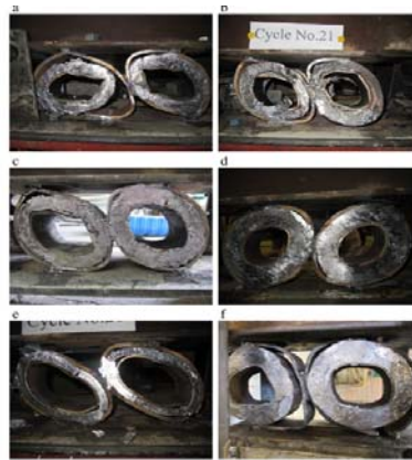
Figure (3): Deformation of tested specimens under cyclic loading
