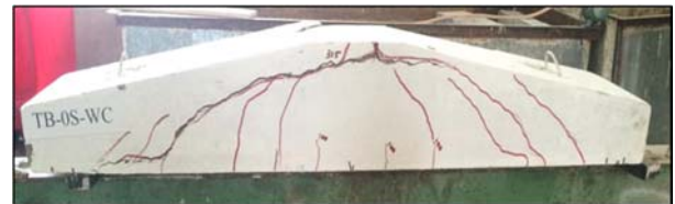
Figure (4): Crack patterns of beam specimen (TB-0S-WC)
