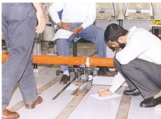
Photo 10: Recording lateral displacements
