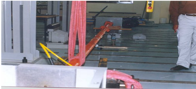
Photo 1: Alignment of the prop between the two supports
