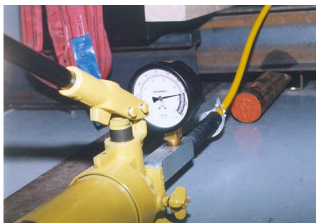
Photo 11: Load (pressure) increasing (=650 bars)
