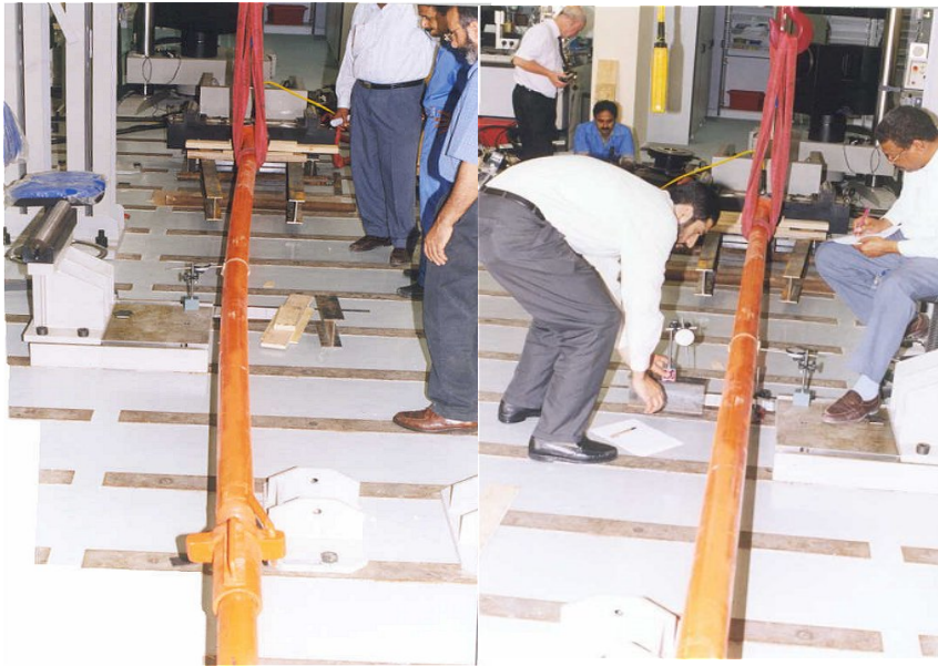
Photo 8: (a) Loaded prop-buckled (b) Unloaded prop-straight
