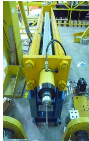
(b) After prestressing (live end hydraulic jack)
