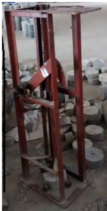
Figure (11): Modified drop impact testing machine
