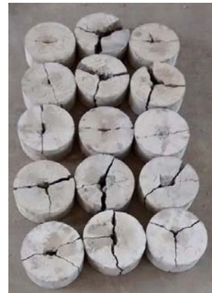
Figure (12): Failure pattern on final impact failure
