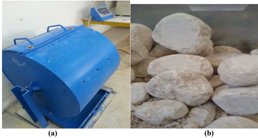
Figure (5): (a) Los Angeles (LA) abrasion testing machine, (b) samples after abrasion
