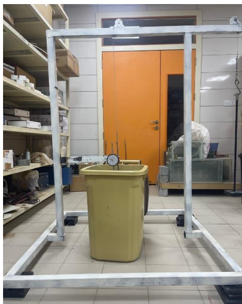
Figure 3. Pullout device and testing tank
