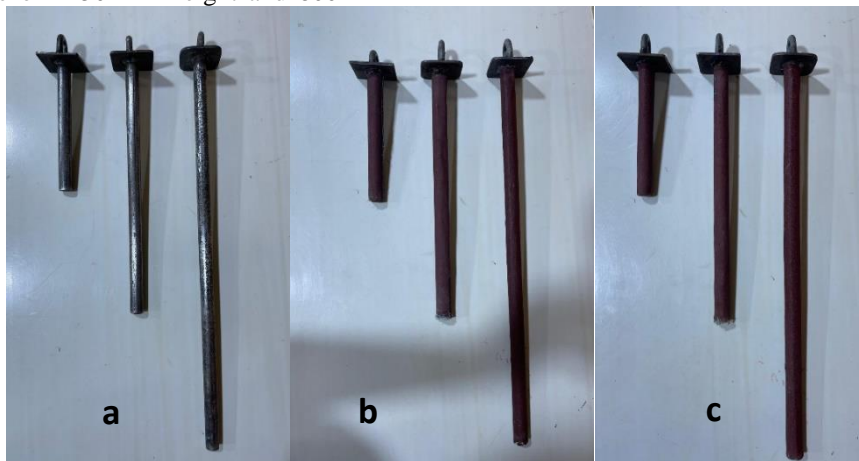
Figure 2. Various geometry ratio (L/D) and skin roughness modeled Piles: a) Smooth skin; b) Medium skin and c) Rough skin
