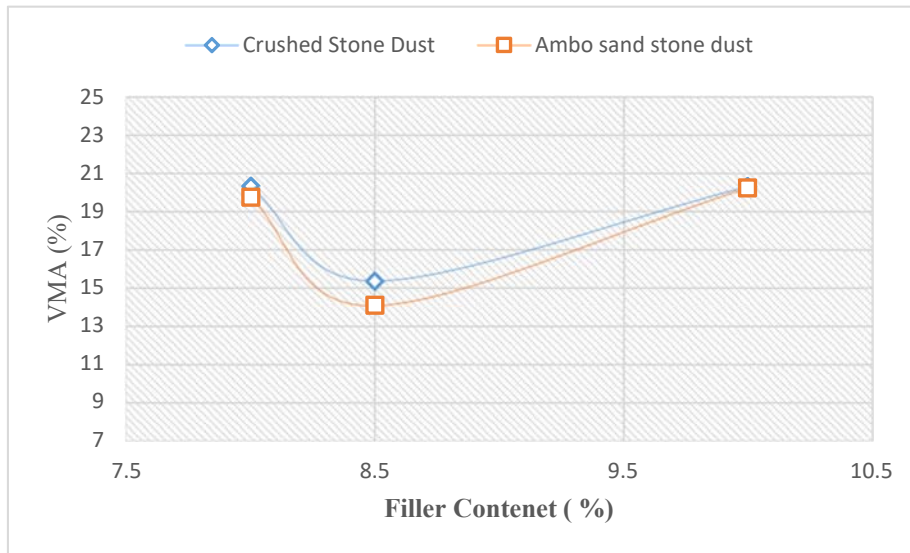
Figure (2): Effect of filler type and content on VMA at OBC
