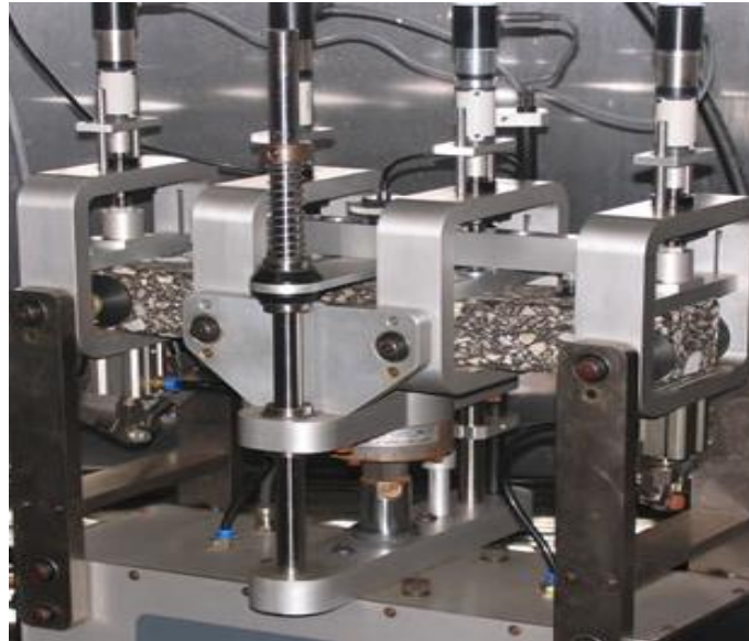
Figure 3. The setup for the four-point beam fatigue test
