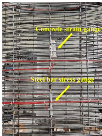
(a) Stress gauge and strain gauge installation
