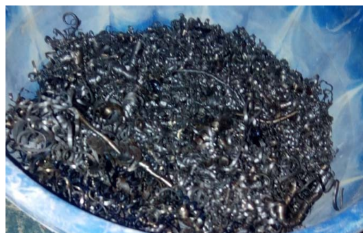
Figure (2): Lathe waste steel fiber
