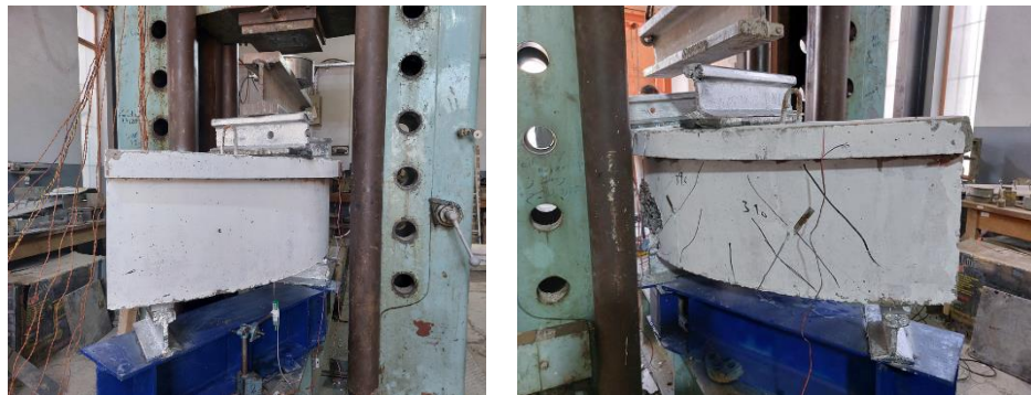
Figure 3. The loading condition, geometry and cracking patterns of box girders
