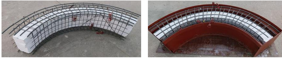
Figure 2. Box girder moulds and reinforcement details
