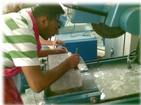
Cutting the Masonry Bricks
