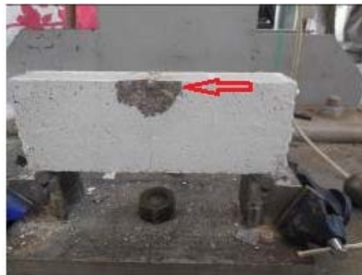
(C) Surface crush
