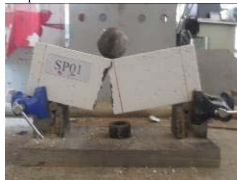
Figure (5): Fracture of specimen SP01-B1
