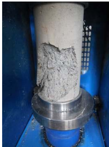
Figure (3): Compressive test set-up
