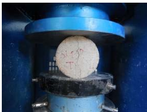
Figure (4): Splitting tensile test setup
