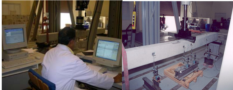
Figure 3: Test setup and the arrangement of LVDTs
