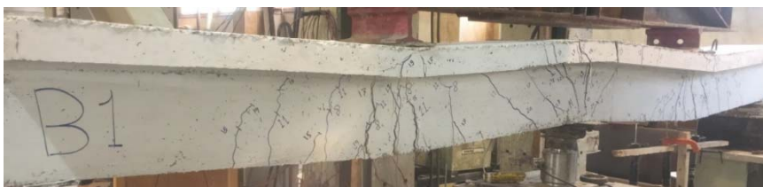
Figure (4): Beam B1 at failure
