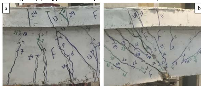
Figure (6): Failure mode of S2 a) at the middle of the span; b) at the intermediate support
