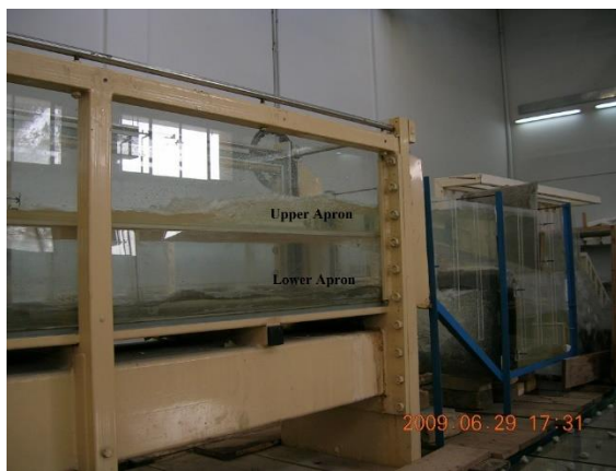
Figure (5): The upper and lower apron along flume from different views and the position of the two-story measuring channel (Bina & Saghi, 2017)
