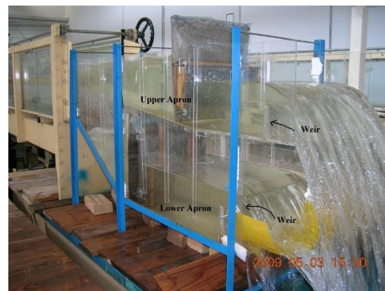
Figure (6): The two-story measuring channel attached to the end of main flume and equipped with two sharp crested rectangular weirs (Bina & Saghi, 2017)
