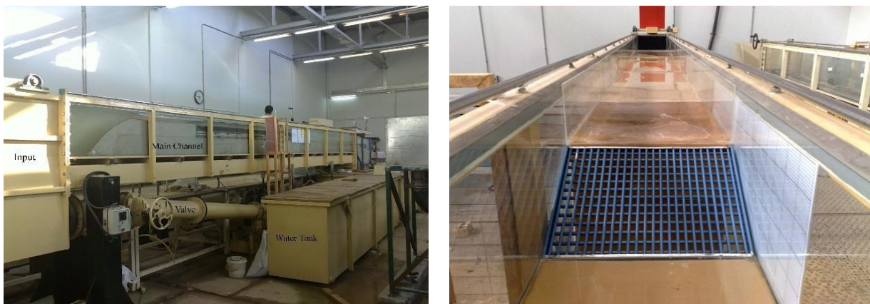
Figure (3): Experimental setup: a) left picture, setup overview, b) right picture, mesh-panel bottom rack, downstream view (Bina & Saghi, 2017)
