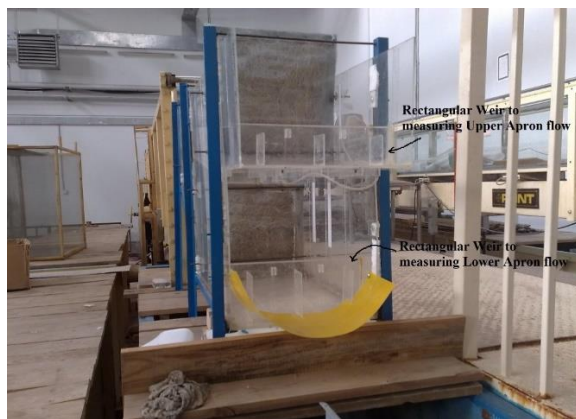
Figure (6): The two-story measuring channel attached to the end of main flume and equipped with two sharp crested rectangular weirs (Bina & Saghi, 2017)
