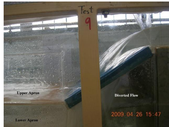
Figure (4): The upper and lower apron and rack position in experimental setup before and during run (Bina & Saghi, 2017)
