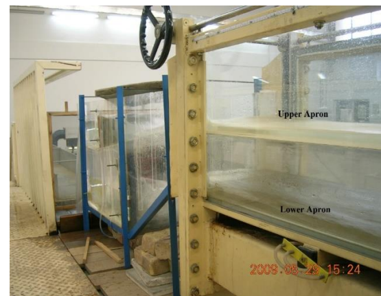
Figure (5): The upper and lower apron along flume from different views and the position of the two-story measuring channel (Bina & Saghi, 2017)
