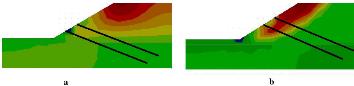
Figure (15): Arrangement of two parallel anchors: (a) x = 2 , and 4 mm; (b) x = 4 and 6 mm
