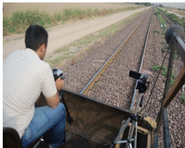
Figure (7): Track survey by car and camera (Tehran-GARMSAR), train speed of 20 to 30 km/h
