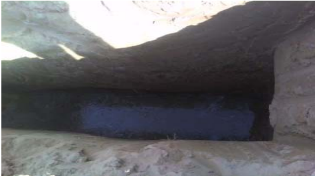
Figure (4): Encountered water table level below 4.5 m depth at the site location
