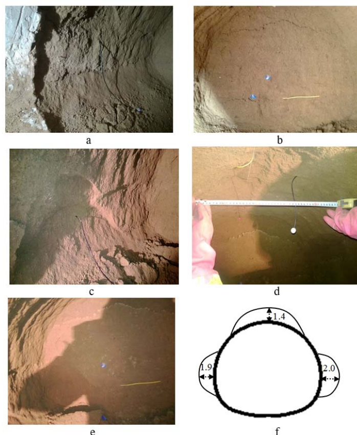
Figure (13): Instability process of tunnel (unit:m). (a) Peeling of sidewall, (b) Transverse crack of excavation face, (c) Collapse of sidewall, (d) Measurement of collapse range of vault, (e) Instability collapse of excavation face, (f) Collapse depth of actual engineering
