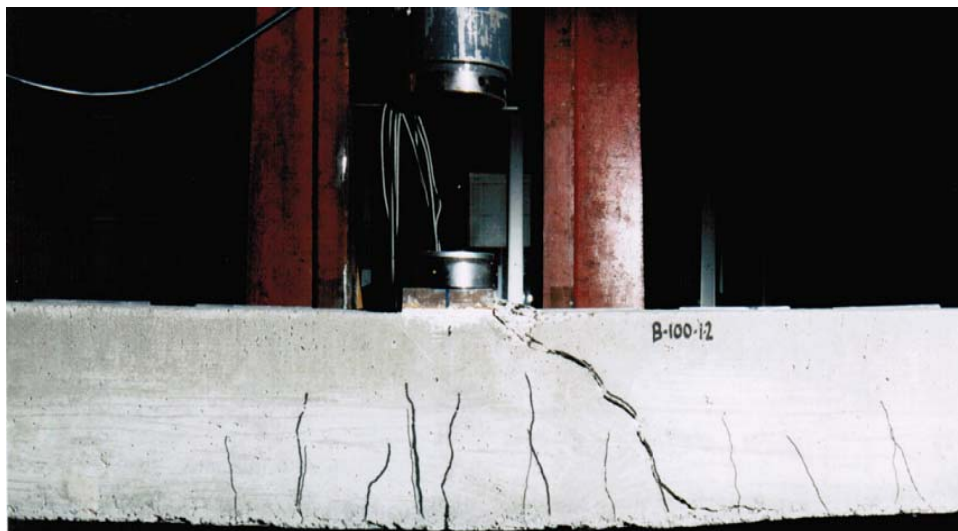
Figure 11: Shear failure of beam 100-12
