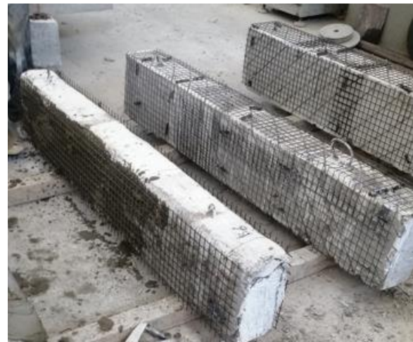
Figure (2): The concrete beams with mesh reinforcement
