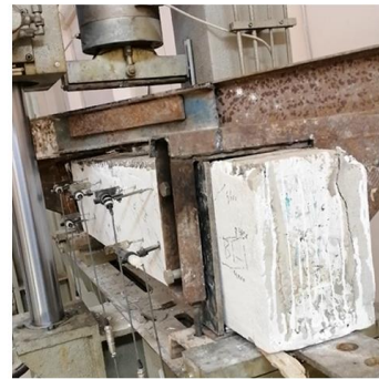
Figure (7): The ineffective separations of the ferrocement laminates in BRS1
