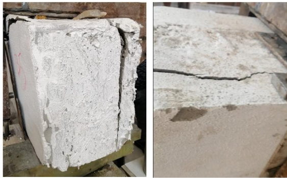
Figure (6): The partial separations of the ferrocement laminates in BRS2
