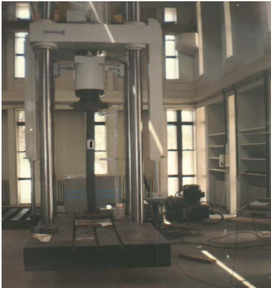
Figure 2: Load Application on Column Specimen
