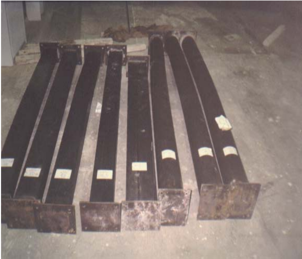
Figure 5: Mode of Failure for Some Tested Columns
