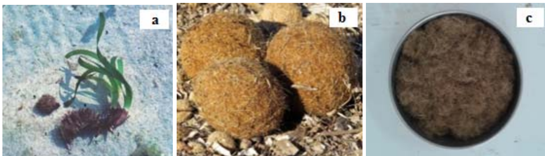
Figure 2: (a) Bundles of Posidonia oceanica leaves, (b) Posidonia oceanica balls and (c) Posidonia oceanica fibers
