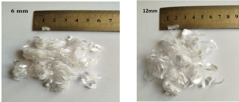
Figure 3. Polypropylene fibers used for the reinforcement
