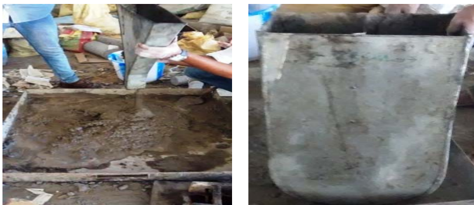
Figure (2): V-funnel and U-box test
