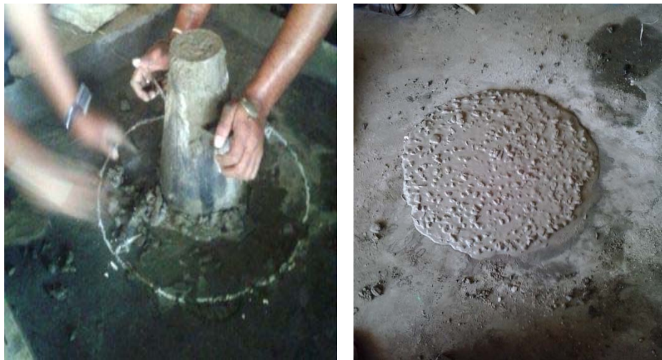
Figure (1): Slump flow and T500 test
