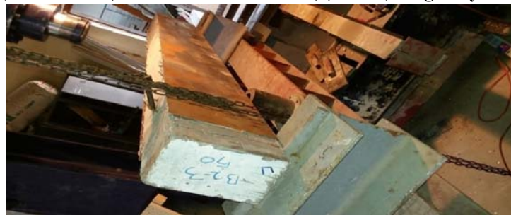
(c) B2-3(U-layer of steel plates)
