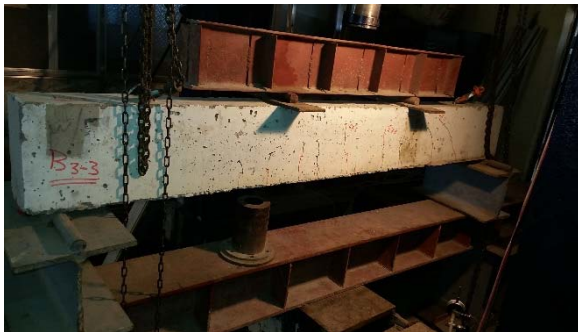
Figure (3): Loading arrangement of the control beam (B1)
