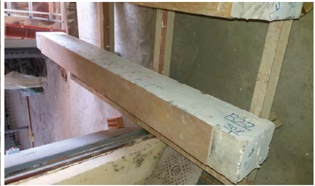
(b) B2-2 (straight layer of steel plates)
