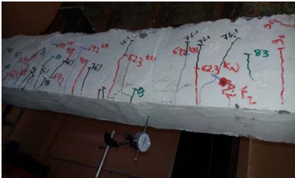
(a) Flexural failure and debonding of ferro-cement layer of beam B2-1
