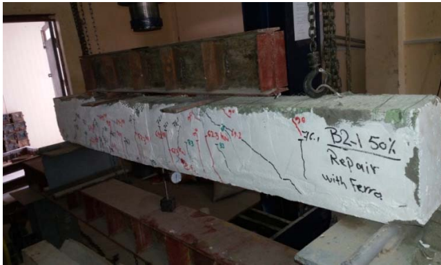
(a) B2-1 (ferro-cement)
