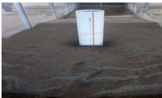
Figure (9): Experimental work showing the pier bridge sample B
