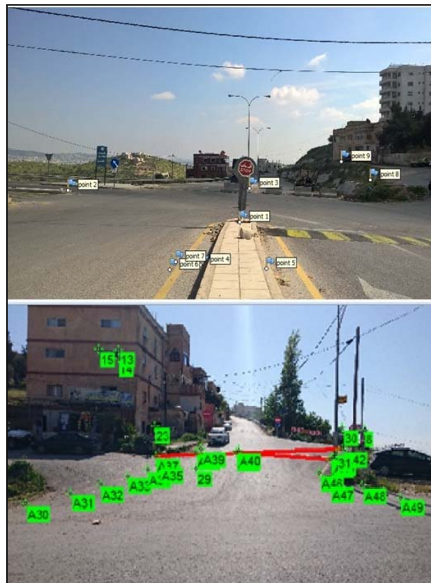
Figure (5): Sample of measured points and objects from the generated surface using iWitnessPRO
