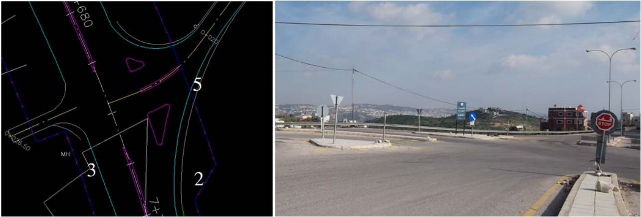
Figure (1): Study area on Salt ring road. Left: generated as-built drawing using total station. Right: image of the study area
