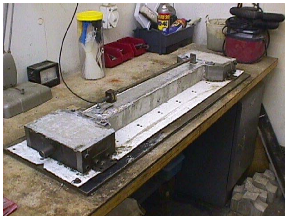
Figure 1: Creep-Shrinkage Test Set-up
