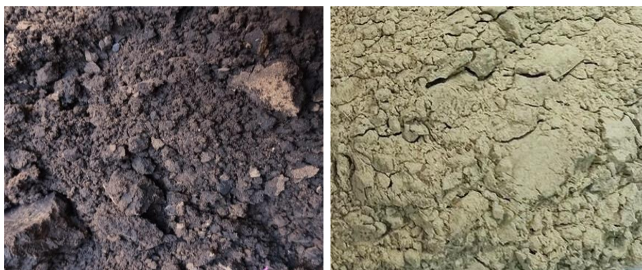
Figure (1): (right) Oily industrial bentonite clay waste, (left) The TRBCW adsorbent in this study
