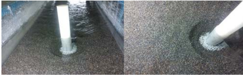
Figure (12): A view of scour hole protected by nano-clay material
