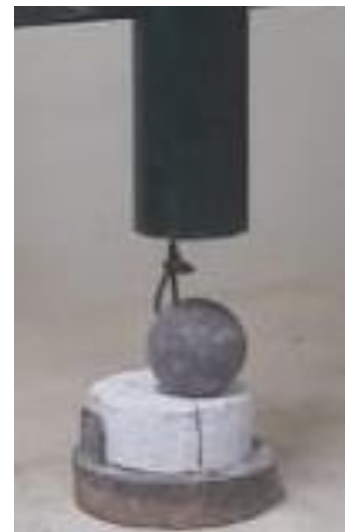
Figure (1b): Specimen details 150 mm diameter & 60 mm height
