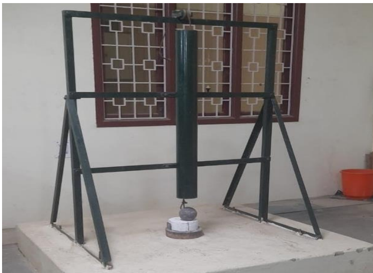
Figure (1a): Drop-weight impact loading test setup
