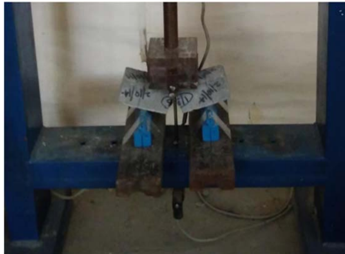
Figure (4): Flexural specimen after failure
