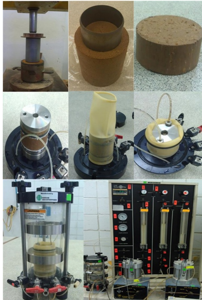
Figure (2): Sample preparation procedure for hydraulic conductivity test
