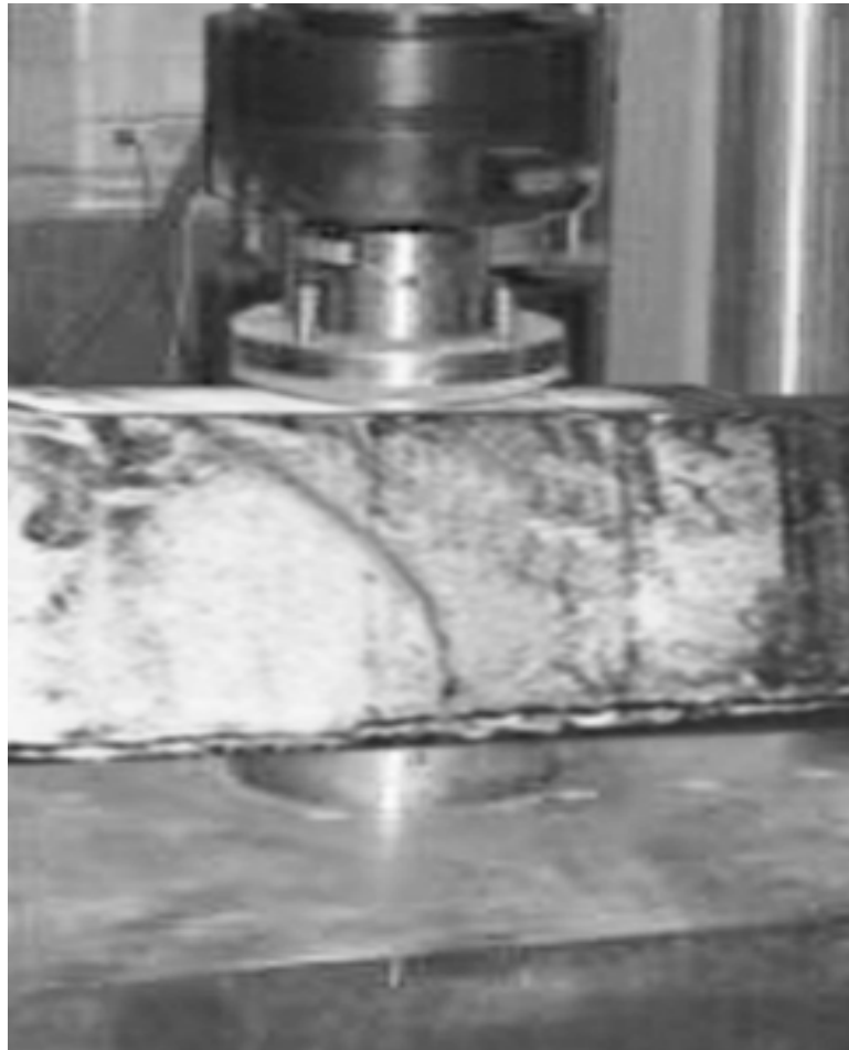
Figure (4): Shear Failure of Beam with GFRP.
