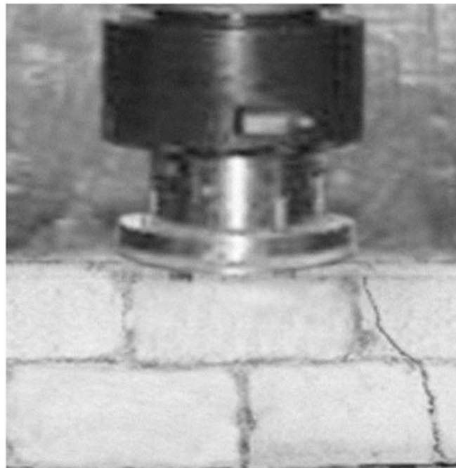
Figure (3): Shear Failure for Beam Tests.
