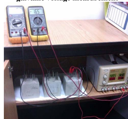
Figure (6): Electrical testing photos showing resistivity measurements
