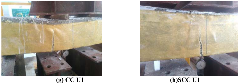
Figure (11): Flexural failure of CC U1 and SCC U1 beams
